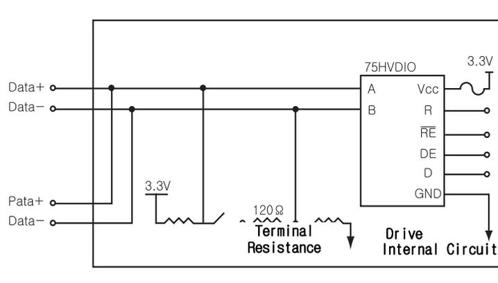
The above figure shows an I/O circuit of RS-485 communication interface signal. When communication is connected, Ezi-SERVO Plus-R maintains to receive stand-by status. It performs sending only when it receives the signal from upper communication and then replies. For more information about communication function, refer to 「[User Manual - Communication Function](#)」 in a separate volume.
