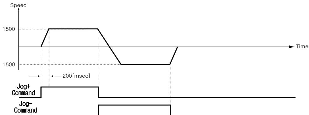
Also, when any value except 0 is set to the 'Jog Start Speed' parameter, the relation between jog command and in-position is shown below.
