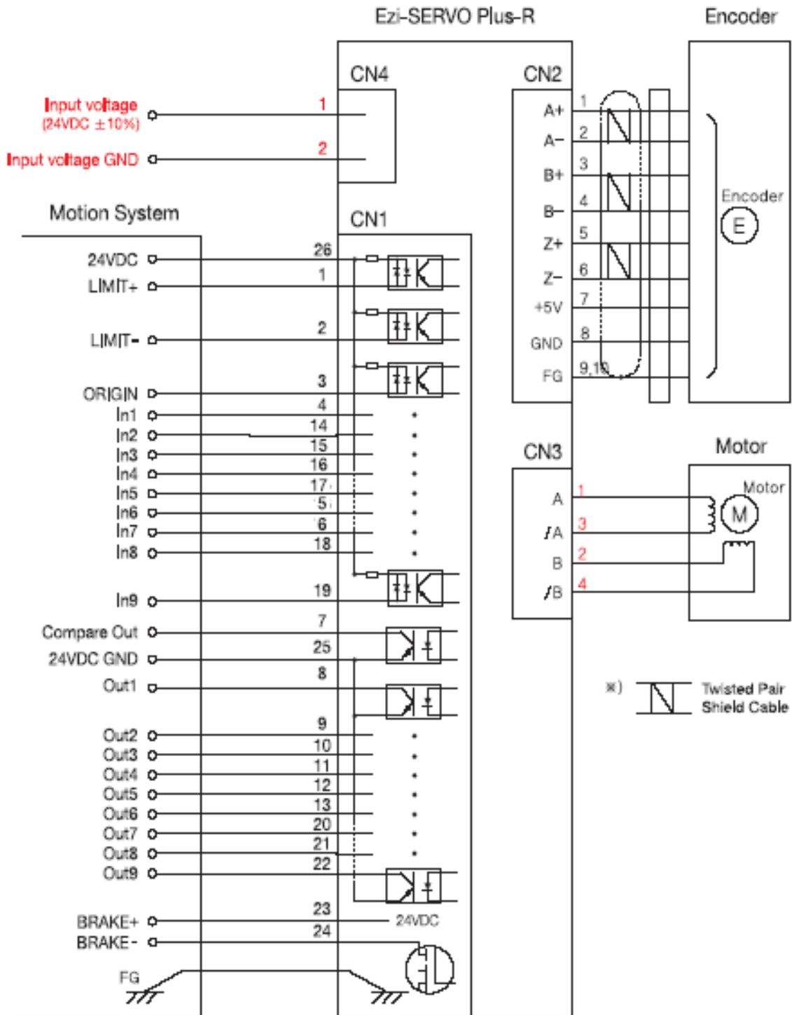
2) Wiring of Ezi-SERVO-PR86
