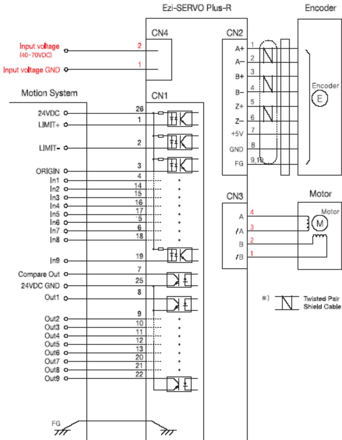
2) Wiring of Ezi-SERVO-PR-MI
