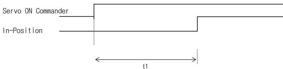
't1' is the time until Servo ON command is given and then the position is decided. It is about 400 msec. It is subject to the rising time of supplying power and the motor status.
