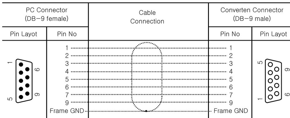
2) Cable of connecting RS-485 Converter and Drive Module(CN5 : Ezi-SERVO-PR only)
