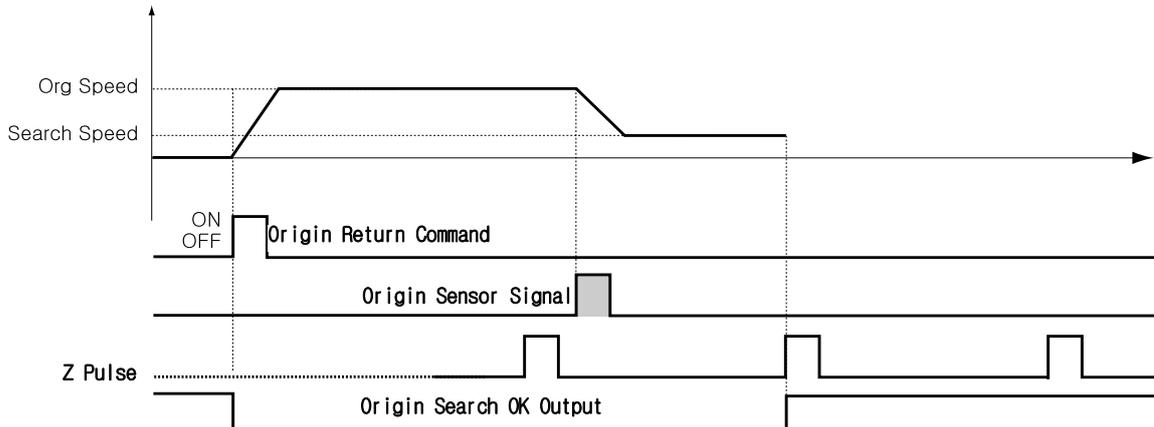
The machine moves up to the origin sensor by 'Org Speed' and 'Org Acc Dec Time' parameters and then completes Z-pulse origin return at the low speed set to 'Org Search Speed'. That is, after the origin sensor is sensed, the machine moves slowly to the original moving direction until Z-pulse signal is sensed.
