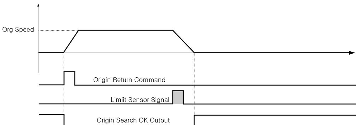
The machine moves up to the position which the limit sensor is sensed by 'Org Speed' & 'Org Search Speed' parameters, and stops by 'Org Acc Dec Time' value. The moving direction complies with as set in 'Org Dir'. If there's no limit sensor on your system, you can set 'Origin' by 'S/W Limit Plus Value' and 'S/W Limit Minus Value' of parameters.
