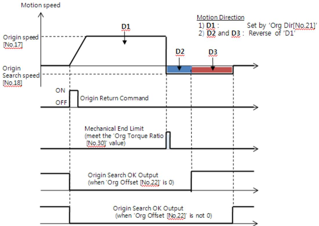
When the machine moves up to the mechanical limit by 'Org Dir' direction, it stop immediately and moves in reverse direction until 'D2' distance. If the 'Org Offset' parameter is not 0, it moves more as 'D3' distance.
