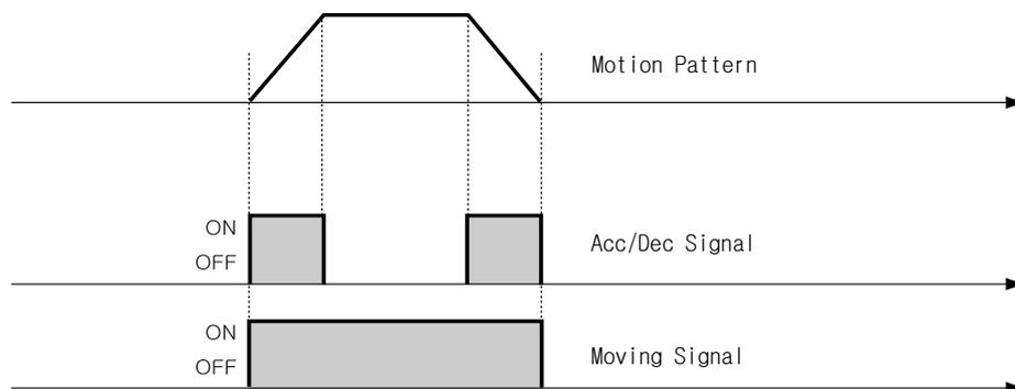
\* Moving signal is not related to actual position. The signal becomes to [OFF] Just after the 'position command' is finished.
