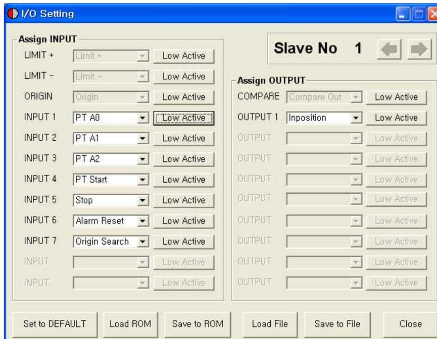
The assignment method is same in input and output.
