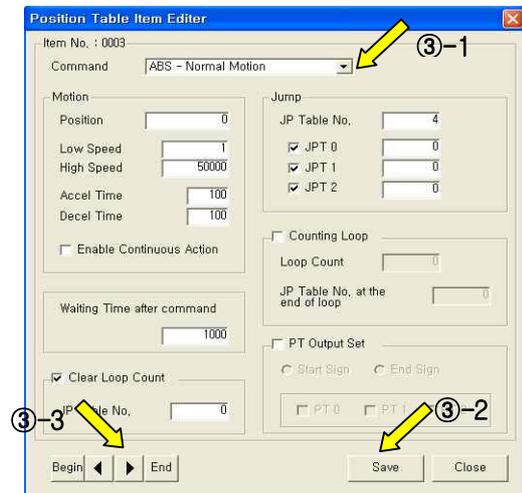
This data is saved to the RAM area. So, when power is off, data is deleted. Click 'Save to ROM' button, and save the data to the ROM area.
