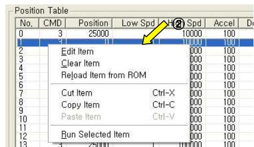
3) Put the mouse on a specific PT data line, double click its left key, and the right window will be displayed.
