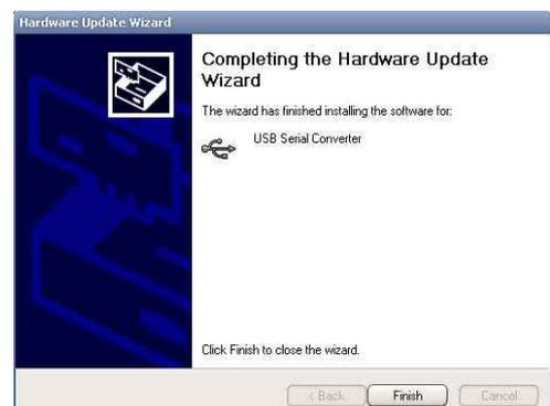
After installation finished, converter can be checked in Device Manager window.
