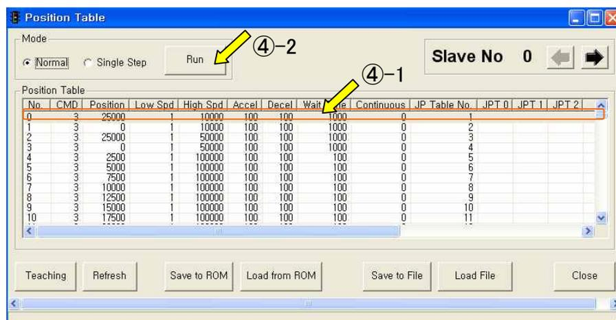
While PT No is operated in sequence, PT lines in service are changed in grey. Also, the user may monitor the operation status as described at '7.3 Position Status' and '7.4 Axis Status' through 'Motion Test' window,
