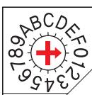
\*Maximum 16 axis can be connected in one network.
