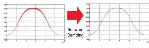
\*This is real measured speed that using 100000[pulse/rev] encoder.
