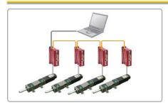
A maximum of 16 axis can be operated from a PC through RS-485 communications, All of the motion canditions are set through the network and saved in Flash ROM as a parameter. Motion Librart(DLL) is provided for programming under windows 2000/XP.
