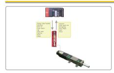
Position Table can be used for motion control by digital input and output signals of host controller. You can operate the motor directly by sending the position table unmber, start/stop, origin search and other digital input values from a PLC. The PLC can monitor the In-Position, origin search, moving/stop, servo ready and other digital output signals from a drive, A Maximum of 256 positioning points can be set from PLC.
